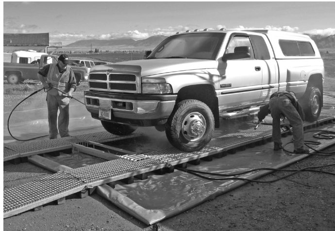
FIGURE 1. Truck being washed by a commercial wash unit as part of the vehicle washing experiments. The truck is driven along the elevated racks while being cleaned by undercarriage washers and hand held pressure hoses.
